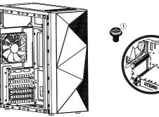
Remove the baffle marked in the picture, make sure the Graphic card aims at the motherboard slot and then fix Graphic card and case with No.1 screw.
