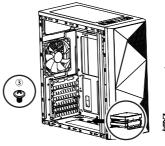
Hard disk enclosure for both SSD and HDD; unscrew hard disk enclosure and install HDD with screws.
